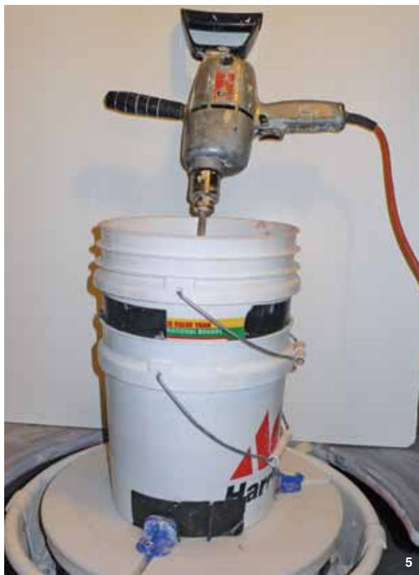
Power sieve (shown from the side) with the drill and the glaze mixing attachment.
