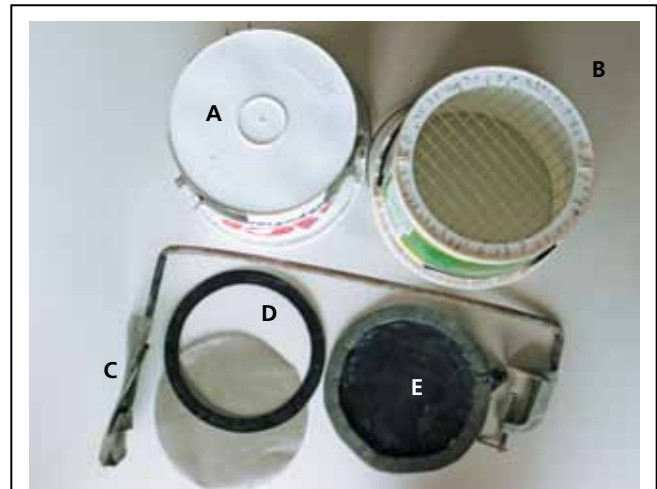
Materials for the power sieve: A—bottom bucket; B—top bucket with ½-inch-square screen (view from the bottom); C—agitator arm; D—stainless-steel sieving screen and sieve screen gasket; E—glaze sealing disk.
