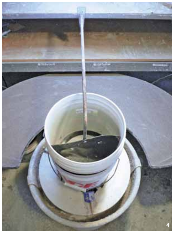
Finished power sieve assembled on the wheel and secured with the Giffin Grip.
