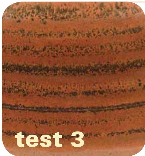
**Cool down: An uncontrolled drop to 1750°F, then -50° per hour to 1600°F, a hold at 1600°F for one hour, then -50° per hour to 1500°F.**
