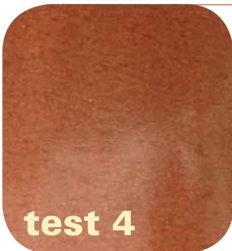
**Cool down: An uncontrolled drop to 1750°F, hold at 1750°F for half an hour, then -50° per hour to 1650°F, hold at 1650°F for one hour, then -50° per hour to 1500°F.**
