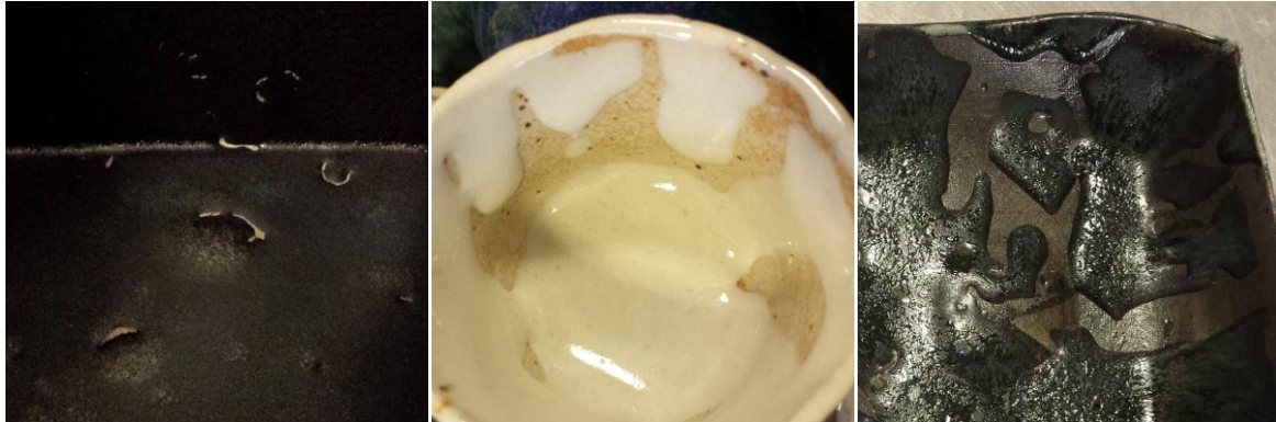
Examples of crawling glazes, from minor to severe.
