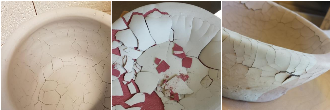
Examples of glaze cracking as it dries due to shrinkage.
