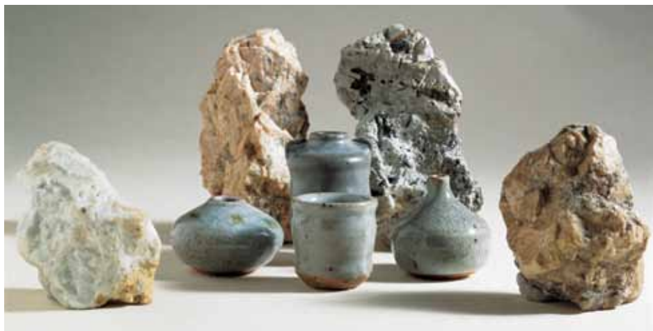
Feldspars and Rocks: Stoneware test pots by Barbara Beck, fired to cone 9–10 reduction. Glaze: Feldspar 90%, Whiting 10%, Red iron oxide, ½%. Pots, left to right: Potash feldspar, Cornwall Stone, Soda feldspar. Pot, rear, center: Nepheline Syenite. Rocks, left to right: Soda feldspar, Potash feldspar, Nepheline Syenite, Cornwall Stone.
